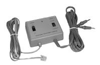
Record all telephone calls automatically as soon as you pick up the receiver. When receiver is hung up, recorder stops. If recording is not desired, turn power switch to "OFF" position. Operation is quick and simple. Insert plugs into cassette recorder and modular plug into No. TEC29 dual adaptor jack and the telephone into the other adaptor jack. (Philmore's No. TEC29 is supplied.)
